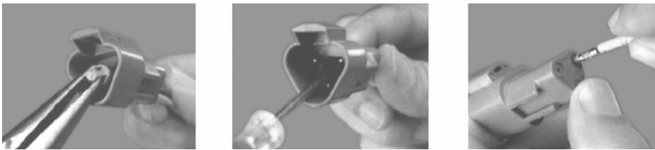
Figure 6-13. DT/DTP Contact Removal
