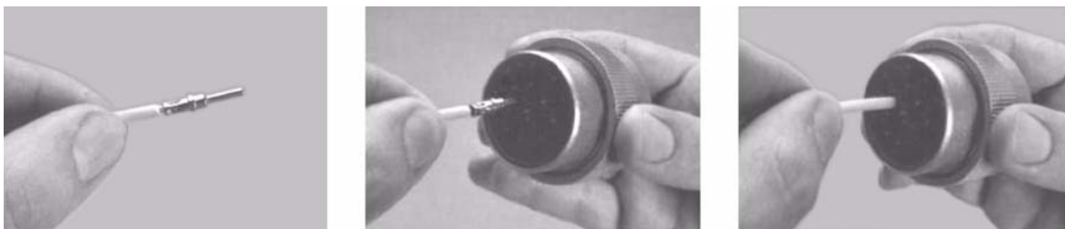
Figure 6-14. HD/HDP Contact Installation
