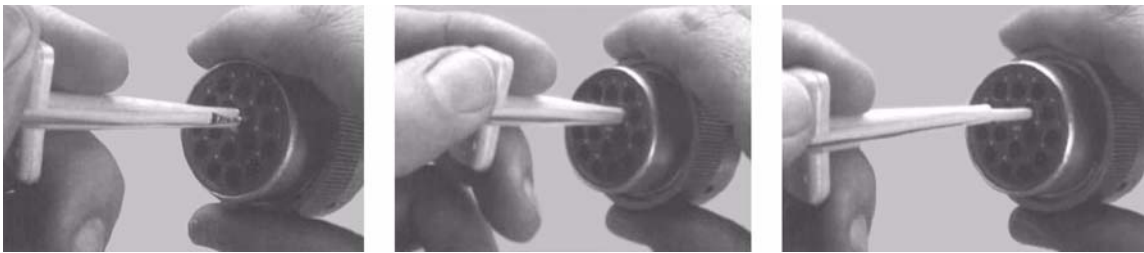
Figure 6-16. HD/HDP Contact Removal
